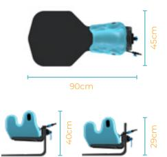
\*The height adjustable head support offers 115mm of vertical range.
